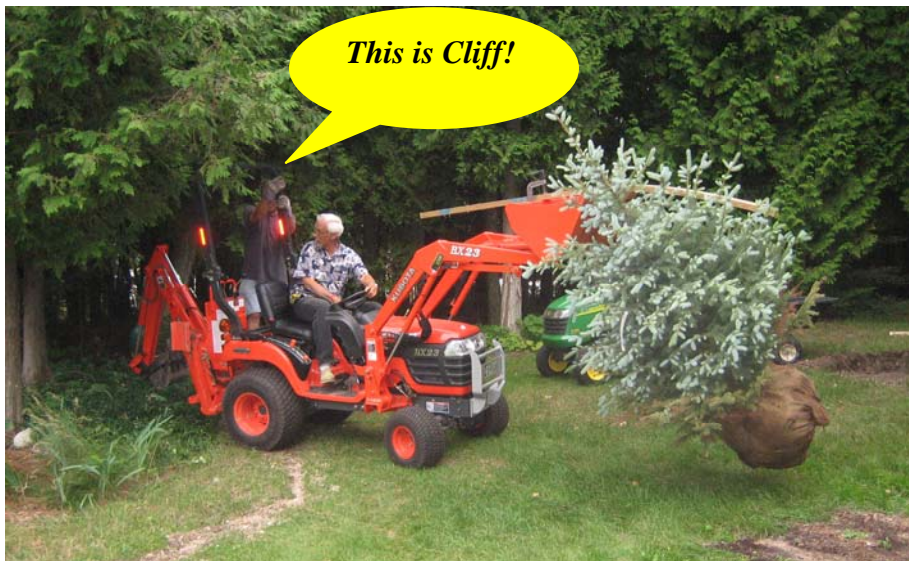
Note the 2x6 boom, (see the bow). Also note the "C" clamps, and our neighbor Cliff, acting as extra ballast on the rear of the tractor to keep it from tipping.
